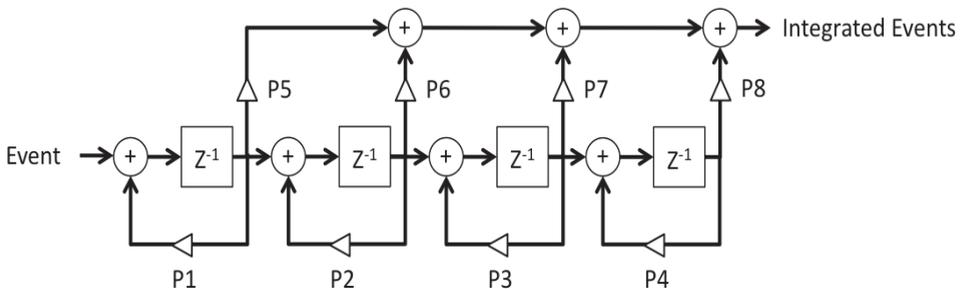
Fig. 10. Filter structure used for integration of evidence.
